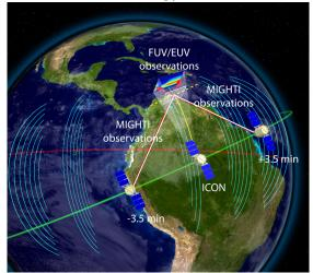
ICON travels eastward and continuously images the thermosphere and ionosphere. Fore- and aft-viewing Michelson interferometers (MIGHTI) measure the vector components of the wind. FUV and EUV instruments make coordinated measurements of the atmosphere and ionosphere near the footpoint of ICON's magnetic field-line. An in situ drift meter measures the ion velocity as a response to electric field on the same field-line.
