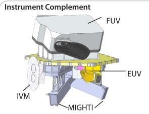
ICON's payload of four sensitive instruments: Michelson Interferometer for Global High-Resolution Thermospheric Imaging (MIGHTI): Remotely measuring the neutral wind field and temperatures - Heritage from SHIMMER flown on STPSat-1.
