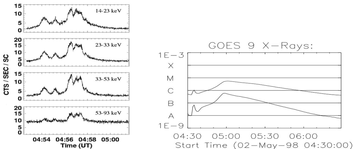
Fig. 2. Left: HXT light curves over all 4 channels showing the impulsive behavior over 4 minutes Right: GOES light curve of the same event, showing the gradual rise and decline of the thermal SXR emission
