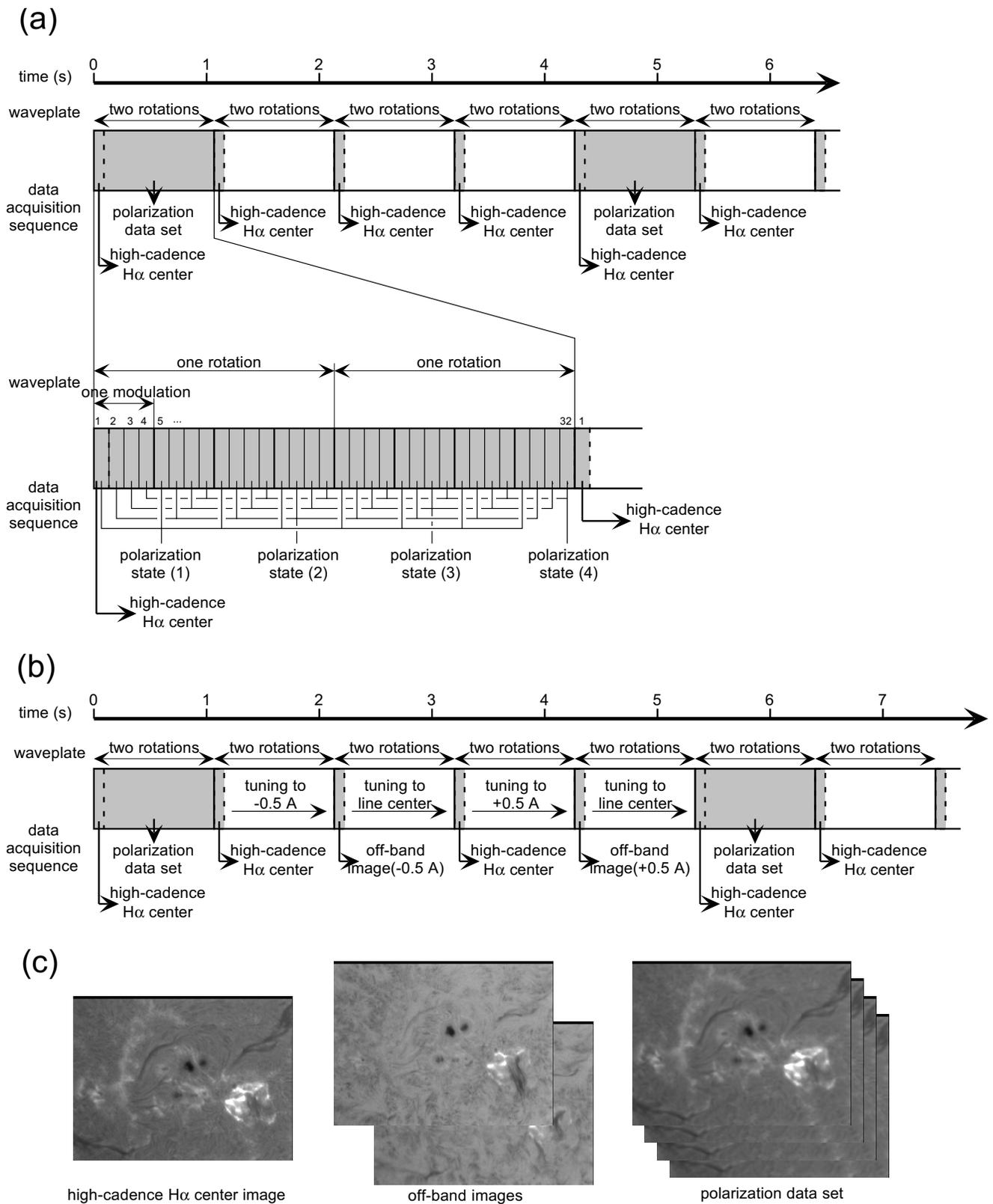
Fig. 2: Time-chart of the data acquisition sequence of the multi-aspect H $\alpha$  imaging system. (a) Basic sequence of the high-cadence H $\alpha$  center imaging and the polarimetry data acquisition. The detail of the polarimetry data acquisition is also shown. (b) Sequence including the off-band imaging for Dopplermetry. (c) Sample images taken with the H $\alpha$  center imaging, the off-band imaging, and the polarimetry data acquisition, respectively.
