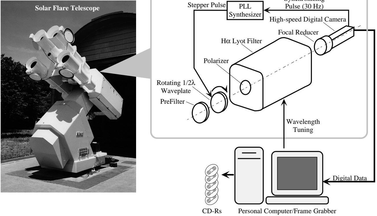
Fig. 1: Schematic drawing of the multi-aspect  $H\alpha$  imaging system. A polarization modulator, a Lyot filter, and a digital camera are installed in one of the refractors of the Solar Flare Telescope of NAOJ, Mitaka.
