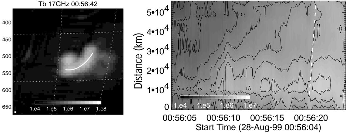
Figure 1: Time variation of the 17 GHz intensity distribution along the microwave ‘loop’ indicated by the solid white line in the left panel. The left lower corner of the loop correspond to the 0 km in the vertical axis of the right panel. Note the propagation around 00:56:20 UT whose speed is  $\approx 9 \times 10^4 \text{ km s}^{-1}$  (indicated by thick white dashed line).
