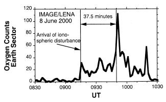
**Figure 3.** Countrate in the Oxygen channels of the LENA imager from the direction of the Earth. A prompt countrate increase occurs at the time of the enhanced proton aurora in Figure 2. A much larger increase in the countrate is seen 37.5 min after the initial ionospheric disturbance.
