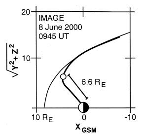
Figure 1. The location of the IMAGE spacecraft in the magnetosphere at the time of a passage of a CME-related shock. The spacecraft was located at approximately 9 LT, 6.6  $R_{\rm E}$  from the Earth. The projection of the magnetic field line from the TY96 model is shown.
