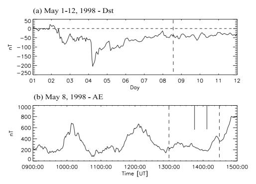
Figure 1. (a) Dst index May 1-12, 1998. (b) AE index May 8, 1998. The dashed lines indicate the time interval we focus on. The two solid lines indicate the onset of the high latitude dayside precipitation events.
