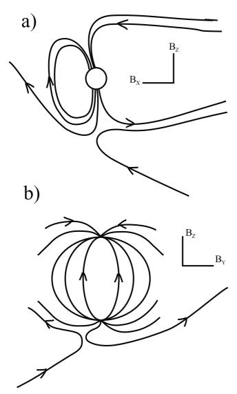
**Figure 5.** Sketch of the field line geometry and merging location when IMF is northward and both  $B_Y$  and  $B_X$  are positive. (a) Meridian scan of the magnetosphere. (b) The magnetosphere viewed from the Sun.
