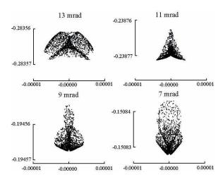
Fig. 13.— Ray trace spot diagrams. Upper left: 13 mrad off axis; upper right 11 mrad; lower left 9 mrad; lower right 7 mrad. Tick marks are spaced 10  $\mu$ m in the focal plane.
