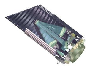
Fig. 11.— Cutaway view of the reference SNAP design. The entire telescope telescope attaches to the spacecraft structure by means of bipods. The outer baffle, shown cut away, also attaches to the spacecraft structure by means of its separate supporting struts. A discardable door, shown open in light gray, protects the cleanness of the optics until on-orbit commissioning begins. Solar panels are fixed, not deployed.
