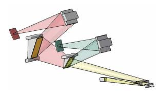
Fig. 17.— A schematic spectrograph optical design. The beam is going out from the slicer (on the bottom right) to a prism disperser back faced coated by a dichroic. The visible light (blue path) is reflected and the IR light (in red) continue to a second prism used to reach the required spectral dispersion. The two beams are therefore focused on two detectors. The dimensions of the spectrograph are approximately  $400 \times 80 \times 100$  mm.
