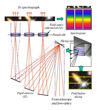
Fig. 16.— Principle of the image slicer. The field of view is sliced along N (here N=3) strips on a slicing mirror. Each slice re-images the telescope pupil onto a line of "pupil mirrors" which reimages the field strip along a "pseudo-slit". The pseudo-slit is placed in the entrance plane of the spectrograph, acting as the entrance slit (courtesy J. Allington-Smith, Durham U.).
