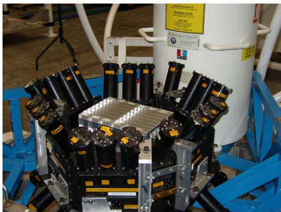
Fig. 4. NCT flight cryostat during integration tests with the BGO shields into the instrument cradle. The entire cradle assembly pivots to allow pointing at different elevations.
