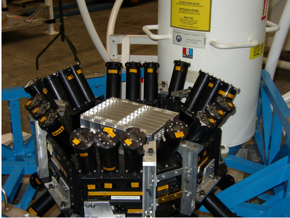
Figure 2. NCT flight cryostat during integration tests with the BGO shields into the instrument cradle. The cradle assembly, including shields and dewar, can pivot to allow pointing at an arbitrary positive elevation.
