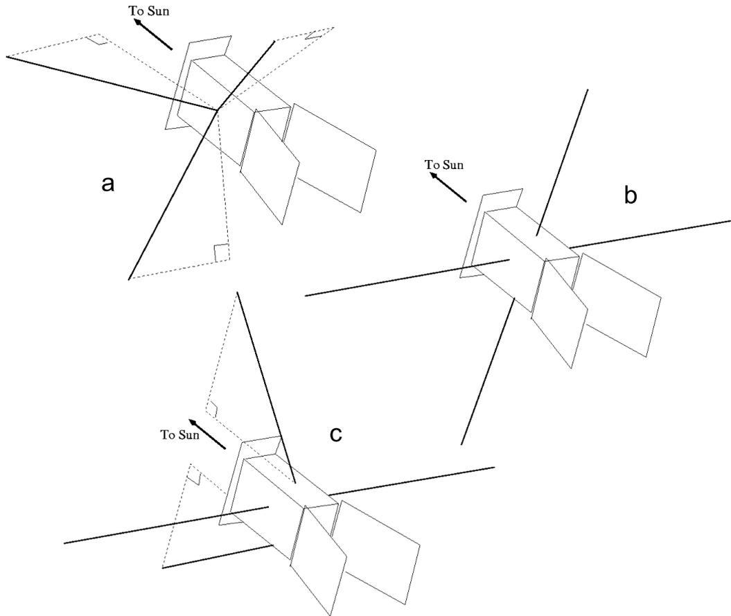
Fig. 4. Some possible Solar Orbiter boom configurations. In each case, the outermost part is used as electric field probes.
