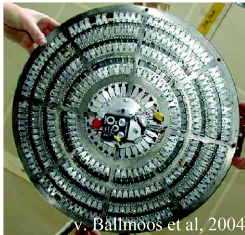
Fig. 4. CLAIRE balloon lens consisting of eight sparsely-populated rings of Ge crystals.
