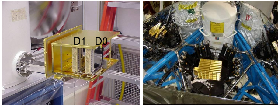
Figure 1. LEFT. The two GeDs, D0 and D1, are attached to a copper coldfinger. Surrounding them on the top and bottom is the partially assembled IR shield. The detectors in this figure are spaced 2" center to center. For the actual flight, the spacing was 1" center to center. RIGHT. The cryostat (gold) containing the two GeDs sits in an active BGO well. In the rear resides the liquid nitrogen dewar. On the sides are pieces of the sun shield.
