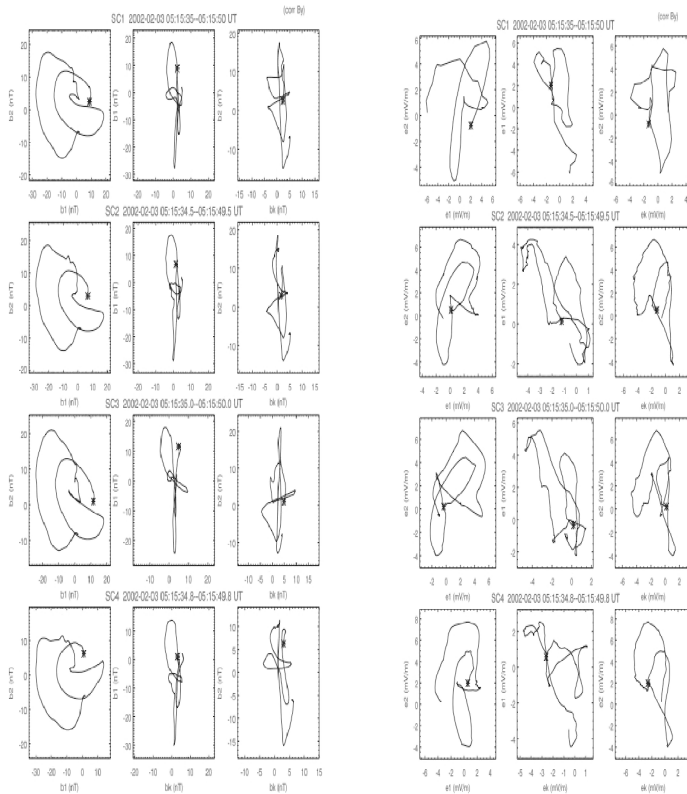
FIGURE 3. Sense of polarization for magnetic (left) and electric (right) fields. The left column of each shows hodograms in the plane normal to \mathbf{k} . The second and third columns are hodograms in the other planes. Observations are shown from the four Cluster spacecraft. The asterisk indicates the start point. Both electric and magnetic fields are right hand elliptically polarized in the spacecraft frame. In the plasma frame, they are left hand elliptically polarized.
