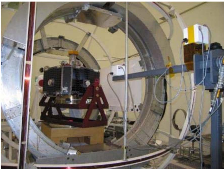
Fig. 7 Showing the coil facility with a THEMIS probe under test. The stand to the right supports the two test magnetometers
