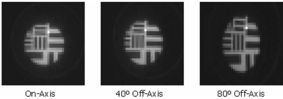
Fig. 22 Typical focus images for the All Sky Imager. A bar test pattern is imaged at various field angles, showing good focus over the entire FOV, although obvious distortion exists off-axis. These are 2X binned images, the normal mode used in the field
