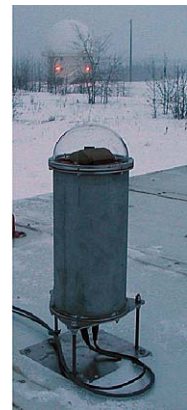
Fig. 6 ASI temperature data from Ft. Yukon. ASI duty cycle is plotted as a temperature 0–10°, corresponding to a percentage of 0–100%. The ASI at Ft. Yukon is shown on the right . A routine period of extreme cold at this location demonstrated the adequacy of the ASI enclosure design
