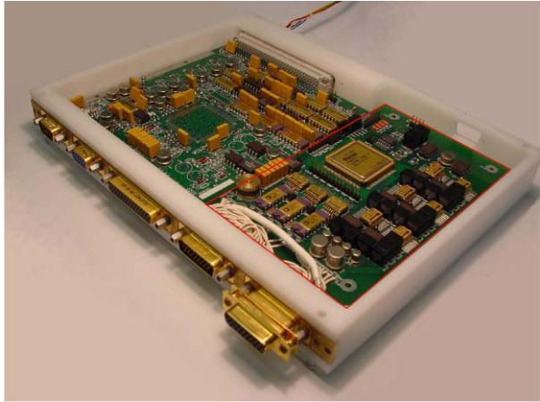
Fig. 6 Themis FGM electronics (red square) placed on a shared board
