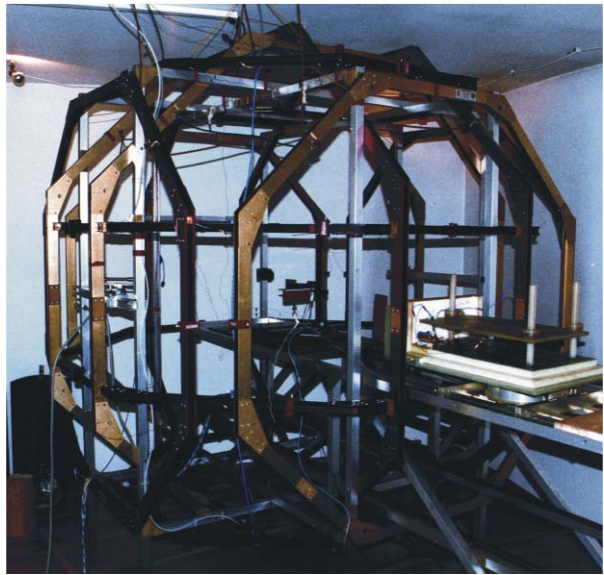
Fig. 16 Coil system with thermal box baseplate in Magnetsrode, Braunschweig
