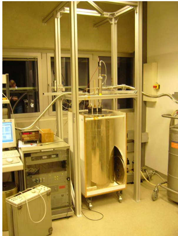
Fig. 13 Facility to measure the dependency of instrument parameters on sensor temperature
