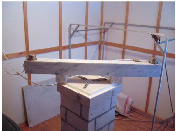
Fig. 17 Two Themis sensors mounted on a pillar to measure Earth field components for comparison with an observatory instrument
