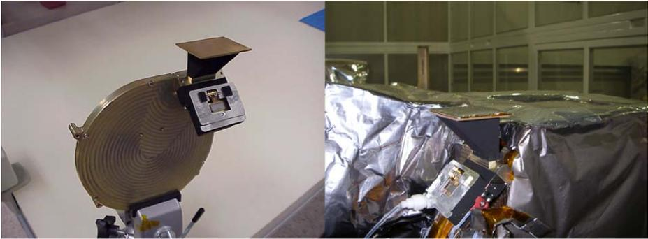
**Fig. 4** STE-U sunshield (*left*) and thermal blanketing (*right*)
