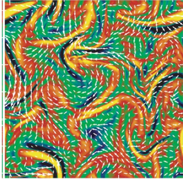
Fig. 5.28 Cross section of the current density along the external magnetic field in color tones. Yellow (light) is positive J_z , blue (dark) is negative and the superposed arrows for the velocity field [47]
