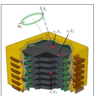
**Figure 3.** Schematic of the WCT (GCT version). By measuring the position and energy of each photon interaction, the initial photon direction can be determined through the Compton scatter formula to within an annulus (event circle) on the sky. Dimensions are  $\sim$ (20 cm)<sup>3</sup>.
