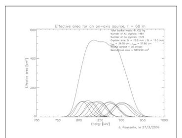
**Figure 8.** Effective area of the LLT. Various sets of Bragg planes in gold and copper at different radii contribute to the broad energy bands. Each Gaussian curve is the contribution of a single ring. The lens achieves ~500 cm<sup>2</sup> for the <sup>56</sup>Co decay (0.847 MeV) from SN Ia.
