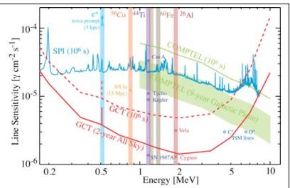
**Figure 6.** GCT narrow line sensitivity  $(3\sigma)$ . The WCT will provide unprecedented nuclear  $\gamma$ -ray line sensitivities, enabling detailed all-sky studies of nuclear processes in supernovae, novae, and other sources in our Galaxy.
