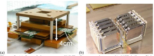
**Figure 5.** (a) Part of the prototype Si/CdTe Compton telescope. (b) NCT balloon flight detectors (GCT prototype), wire-bonded in their cryostat mounting (each GeD is 8×8×1.5 cm<sup>3</sup>).
