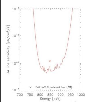
**Figure 9.** Sensitivity of the LLT/WCT combination on DUAL ( $10^6$  sec), enabling study of SNe Ia out to ~50-80 Mpc, for dozens of potential targets each year.
