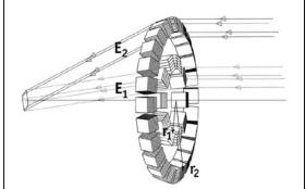
**Figure 7.** Principle of a crystal diffraction lens in Laue geometry  $(E_2 < E_1)$ .
