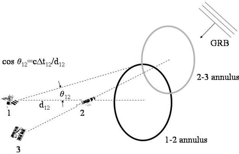
Figure 13.1: The triangulation method. A plane wave resulting from a  $\gamma$ -ray burst is incident on three spacecraft. The difference in arrival times between spacecraft 1 and 2 defines an annulus of possible arrival directions. A third spacecraft gives a second annulus which generally intersects the first one to define two possible arrival directions.
