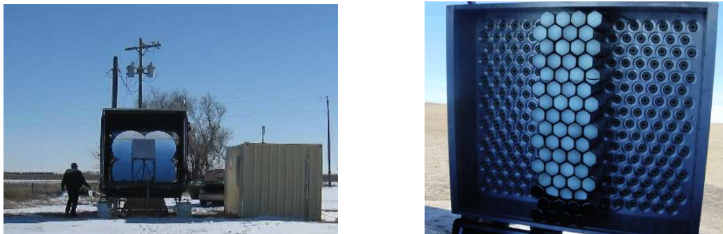
Figure 4: The remotely operated Atmospheric Monitoring Telescope (left) and its camera (right) with the central 4 columns instrumented. A rectangular UV transmitting filter (not shown) normally covers the camera surface.
