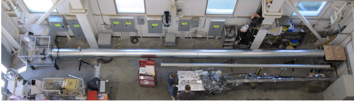
Figure 4. Bird's eye view of the X-ray beamline in the high bay at SSL. The X-ray generator is enclosed in a lead casing on the right hand side of the room (wooden boards) and the Laue lens assembly station is in the plexiglass enclosure on the left hand side of the room.
