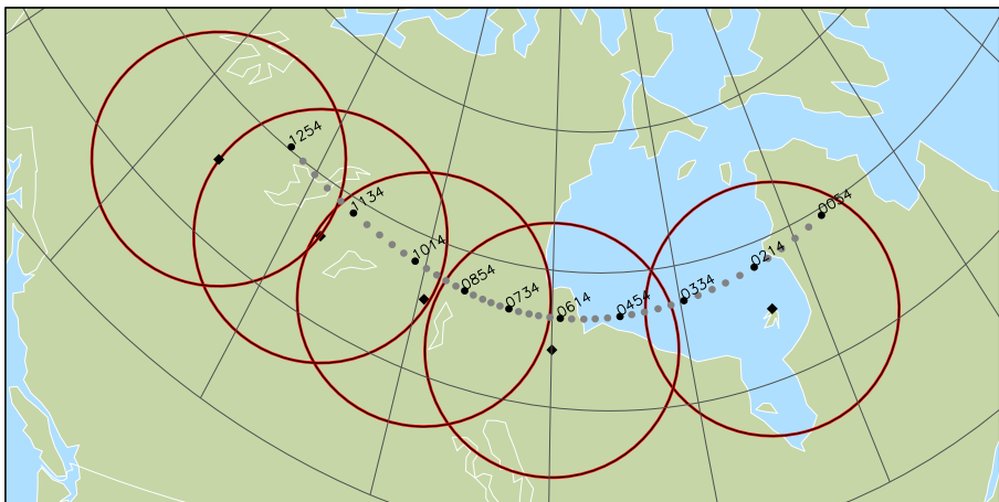
Fig. 14 EIDOSCOPE magnetic footprints superposed on a map showing fields of view of all-sky cameras. The dots are separated by 16 min, with every 5th point highlighted and its corresponding UT shown (courtesy Eric Donovan)
