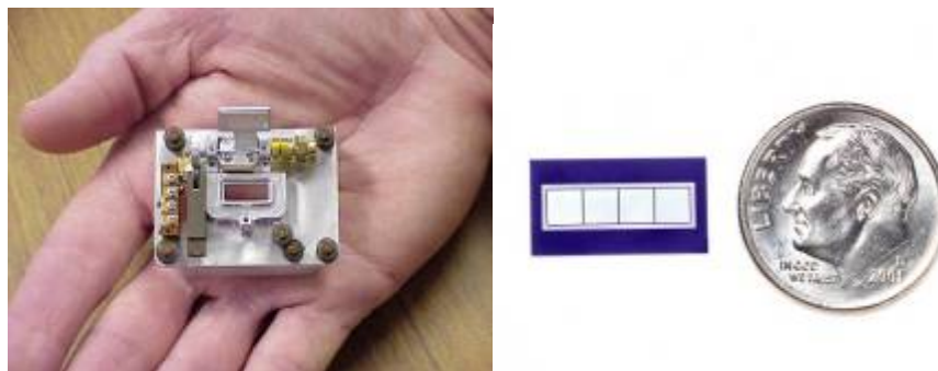
Figure 3. Left. SupraThermal Electron (STE) sensor (engineering model) for NASA's STEREO mission. Right The four pixel (each 0.1 cm 2 ) SSDs with guard rings used in STE.
