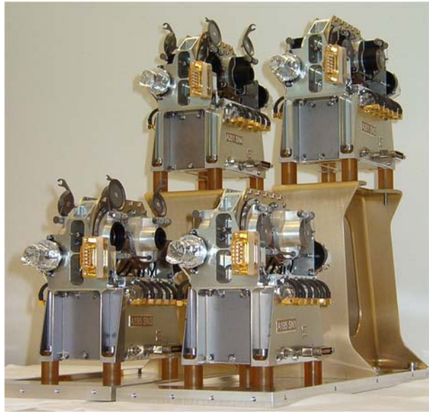
Fig. 1 SEPT-E ( in front ) and SEPT-NS ( on bracket ). SEPT for Ahead S/C with doors closed ( right ), and for Behind S/C with doors open ( left )
