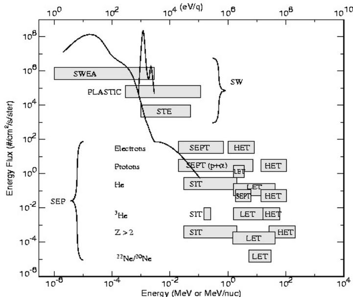
Fig. B.2 The energy and flux coverage of the STEREO IMPACT particle detectors and the UNH-PLASTIC instrument.
