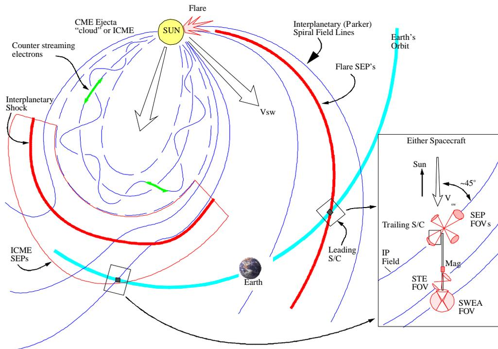
Fig. B.1 The measurement and science domain of the STEREO IMPACT investigation. IMPACT detects solar wind plasma electrons, including the heat flux electrons that can be used to trace magnetic field connections to the Sun, the local magnetic fields, and energetic ions and electrons generated at the Sun in flares and at CME-generated interplanetary shocks.
