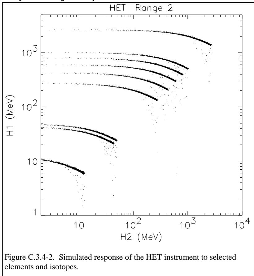
Figure C.3.4-2. Simulated response of the HET instrument to selected elements and isotopes.
