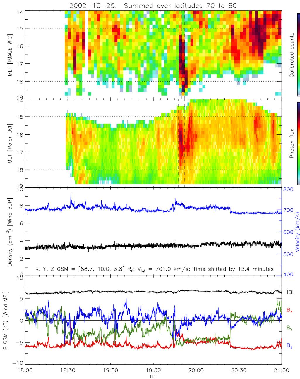
Simultaneous widespread brightening at 19:47 UT in both hemispheres
