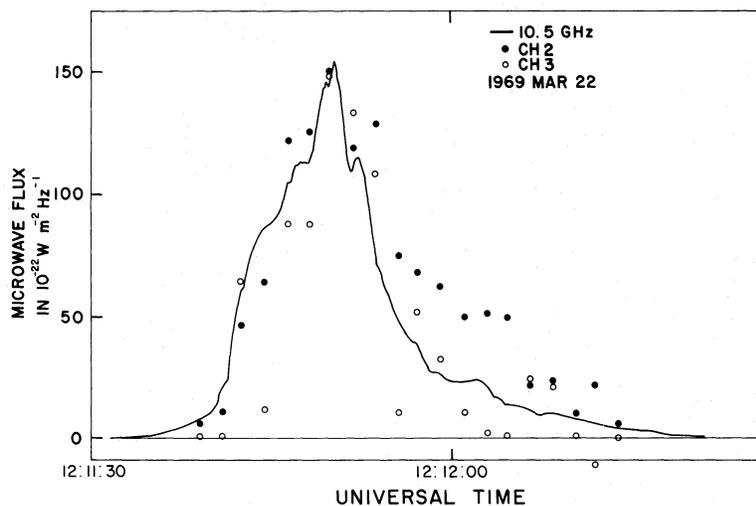
FIG. 2.—The time profiles of the X-ray flux in channels 2 and 3 and the 10.5 GHz flux (Institute of Applied Physics, University of Bern), each normalized to the same peak height, for event number 5.
