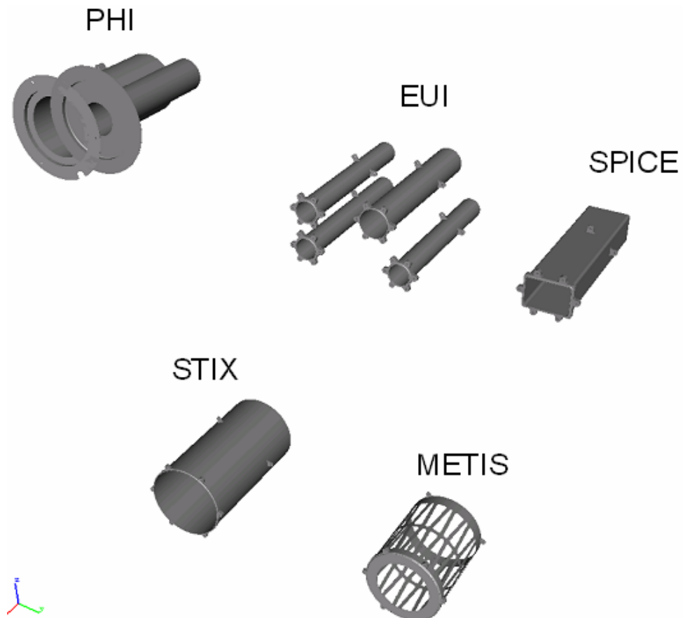
Figure 9 Conceptual Design of Remote Sensing Instrument Feedthroughs
