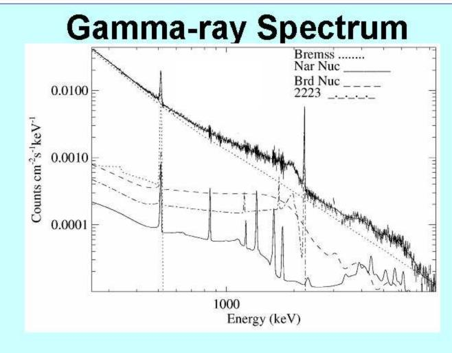
Modeling the observed gamma-ray count spectrum (top) can identify its individual components:
