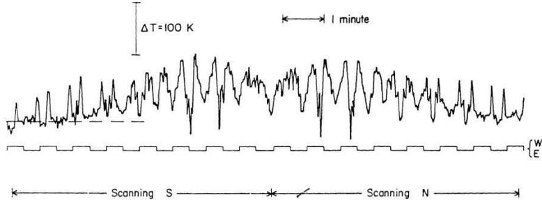
Figure 1: Strip-chart recordings of  $20\mu$  photometry of a solar active region made with the Mt. Lemmon 60-inch telescope through one layer of “Black Polymulch” (like bin-bag black poly). The successive lines of the scan show repeatable features identified with faculae (if bright) or sunspots (if dark).
