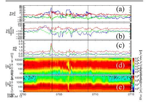
**Fig. 12** TH-E data in identical format as Fig. 11. (a) Magnetic field (nT, LMN: *blue*, *green*, *red*); (b) Partial ESA velocity (km/s, LMN); (c) Magnetic (*blue*), plasma (*green*) and total (*red*) pressure (nPa); (d) and (e) ESA ion and electron omnidirectional e flux ( $eV/(cm^2 \text{ s str eV})$ ). *Dashed lines* denote, again, timing of FTE centers on TH-C, observed slightly earlier on TH-E
