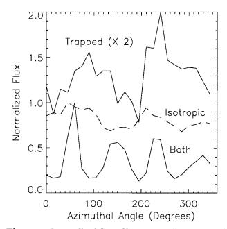
Figure 1. Normalized flux of low-energy (15 to 200 eV) electrons versus azimuthal angle for selected distributions. All of these distributions were measured on July 24, 1992. The "both" (trapped/field-aligned) distribution was measured at 0200 UT; the "isotropic" distribution at 1000 UT; and the "trapped" at 1530 UT. The "trapped" distribution has been multiplied by 2 for clarity.
