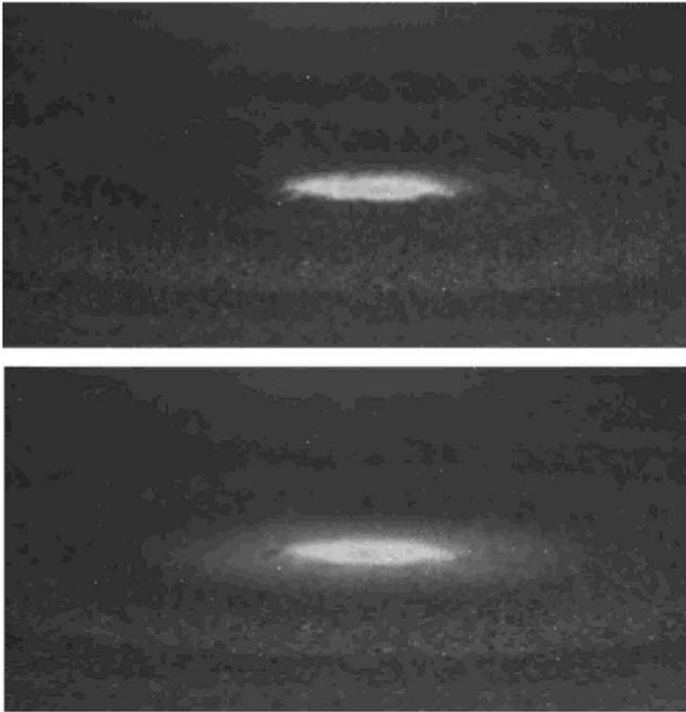
**Fig. 4.** Oblique views of JSC-Mars-1 dust on a graphite plate taken before (top) and after (bottom) the plasma was generated in the plasma device. A broad halo of dust surrounds the original dust spot location after only a few minutes exposure to plasma. The final distribution of dust is stable and no further spreading occurs.
