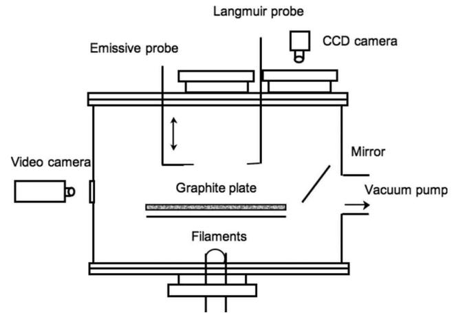
**Fig. 3.** Schematic diagram of plasma device configuration used for horizontal dust transport experiments and electric field measurements
