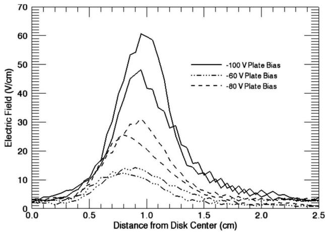
**Fig. 6.** Horizontal electric field determined by taking the derivative of the horizontal potential scans in Fig. 5. The electric field increases as the plate voltage increases and is positive, meaning the field is directed radially outward. The spreading of dust seen in Fig. 4 means the particles are positively charged.
