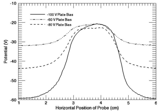
**Fig. 5.** Probe sweeps over an insulating glass disk on a graphite plate in a plasma sheath for graphite plate bias potentials of  $-60$ ,  $-80$ , and  $-100$  V. The sheath potential beyond the edges of the disk varies with the surface potential, but the insulating disk, a proxy for a layer of lunar dust, reaches the same potential regardless of the underlying surface potential.
